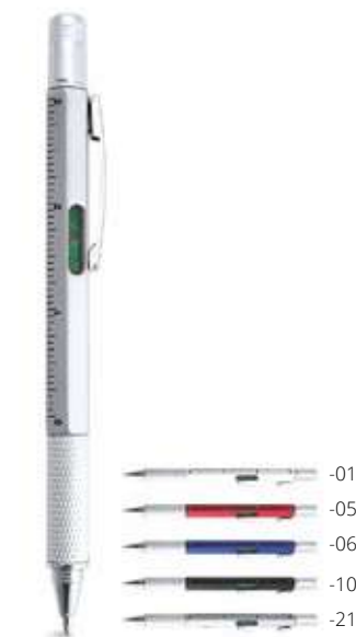
Sauris AP741722 Plastic ballpoint pen with flat and star-head screwdrivers, spirit level and 7 cm / 3 inch rulers. With metal clip and blue refill. Size: ø10×149 mm Printing: P1(2)
